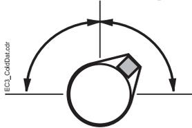
Both air temperature sensors should be mounted on spacers in the air duct so that there is airflow around.
