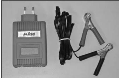
Charge the battery immediately if it is empty when you start the motorcycle. If left to stand in an uncharged condition for a longer period of time, the battery will run down and sulfatize, destroying the battery.
