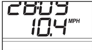
display will change from one mode to the other every few seconds. The lower half of the display will also show your heart rate when you use the handgrip pulse sensor (see step 5). Note: When a program is selected (except for pulse program 1), the display will show the time remaining in the program instead of the elapsed time.
