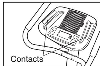
Next, hold the handgrip pulse sensor with your palms resting on the contacts. When your pulse is detected, the heart-shaped indicator in the lower half of the display will flash each time your heart beats, and your heart rate will be shown.
