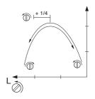
**CAUTION!** If the cutting attachment rotates when the engine is idling the idle adjustment screw T should be turned anticlockwise until the cutting attachment stops.
