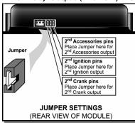
Remote car starters of this series are equipped with an on-board high-current programmable 5th relay that can be used to power a second ignition, accessory or crank wire. The unit uses 3 sets of pins; each set corresponds to a specific function of the output. In order to activate one of the three possible functions, you must place the jumper (supplied) on one of the three sets of pins and connect the 14 AWG wire to the second IGN. / ACC. / CRANK wire of the vehicle.
