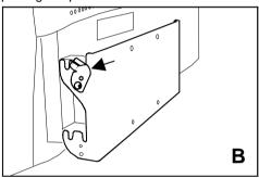
Step 3: Place the panel on the mounting plate
