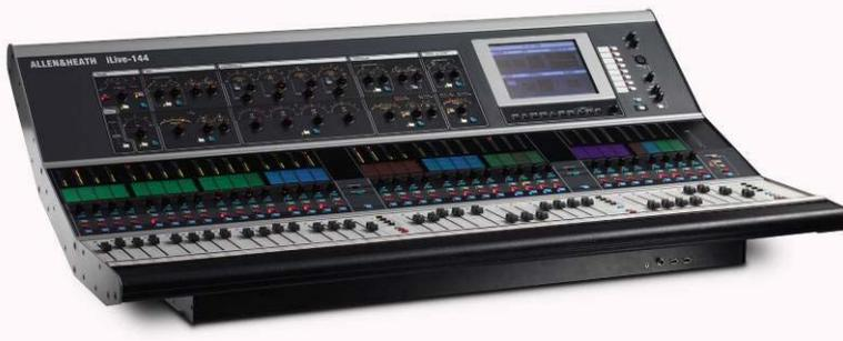
**iLive Surface** There are 4 sizes of control surface available with up to 44 faders. These are arranged in banks with 4 layers each. The surface has a 4 slot card frame built in to load up to 4x 8 channel input or output modules for local I/O.
