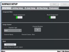
**SURFACE SETUP** Enters a setup mode to use the strip **SEL** keys to assign the Surface strips as input channels, mix masters, DCA masters and more in any combination. You can assign single strips or a range of strips within a fader bank. Other pages let you configure the SoftKey functions, PL devices, the ALT VIEW key, and Surface preferences.
