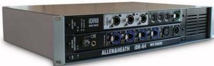
**iDR0 MiniRack** The MiniRack is similar to the iDR10 MixRack except it does not have any card slots for input or output modules. Instead it gets its audio via the EtherSound network. It can be used as the slave mix engine in an FOH/Monitor system with digital mic split, or as a compact mixer with an iLive Surface using the audio I/O in the back of the Surface.
