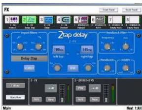
**FX** Access the FX rack. Provides 8 virtual 'rack positions' for loading your choice of processing from a library of effects devices including reverbs, delays, modulators and more. A Front Panel view presents a familiar control interface for parameter data entry. A Rear Panel view lets you 'patch' the device into the signal path either as a 'mix>return' or 'insert'. Choose the input to the device from a mix or direct output, and its output to an FX (short) return or full channel.
