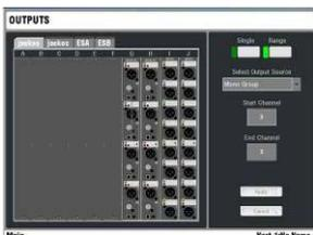
**OUTPUTS** Map signals to the physical sockets and audio network channels. Touch tabs let you select the MixRack, Surface, Port A and B patch bays. Assign single or a range of sockets from a choice of mixes, direct outs, insert sends and other sources.
