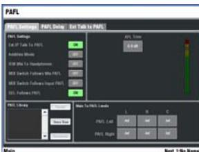
**PAFL** Set user preferences for the PAFL engineer's monitoring system. Choose between additive and auto-cancelling operating mode, adjust the AFL trim to avoid big level differences between PFL and AFL, set main mix to monitor level when no PAFL is selected, and choose to link the SEL and/or MIX keys with PAFL key presses. You can turn on and select the External Input to PAFL source for reverse talkback, and set delay to time align the monitor to the acoustic sound from the stage.
