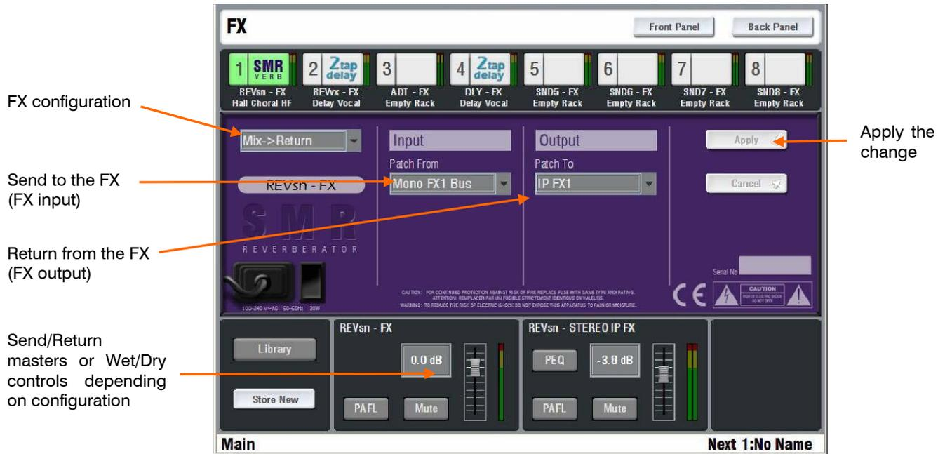
Touch the top right Back Panel button to open up the connections view. This emulates patching up a typical outboard effects rack. Configure the FX device as a send/return loop or inserted into a channel or mix signal path.
