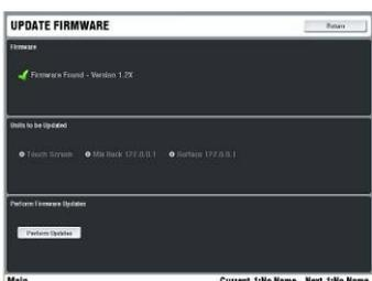
**How to update the system firmware** The downloaded file is extracted to a USB key which is then plugged into the surface for the update to be performed. The MixRack, Surface and TouchScreen are all updated at the same time.
