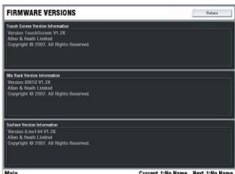
**Firmware Versions** Displays the current firmware versions for the TouchScreen, Surface and MixRack. They should all be the same version. If not the system would fail to connect and would prompt you to view and update its firmware during the boot up process.
