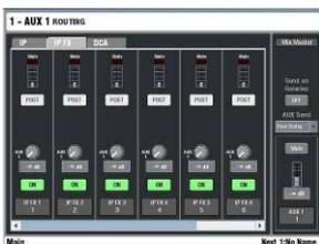
**ROUTING** This screen displays the routing and DCA assignments, direct out trim, send levels and preferences for the channel currently selected using the **SEL** key. For the Aux masters it lets you select the channel send source and choose to have the sends on faders or rotaries. The screen can provide an alternative to adjusting the mix sends and assignments on the fader strips using the **MIX** keys.
