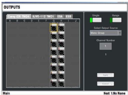
**MixRack** The tab displays the user name assigned to the MixRack. The system identifies the output modules currently loaded (iLive) or fixed sockets available (T Series) and displays a physical socket view. Touch a socket to view its current assignment. Choose a source from the drop down menu, highlight the Channel Number box and use the encoder to scroll through the channel numbers. Touch Apply to confirm.
