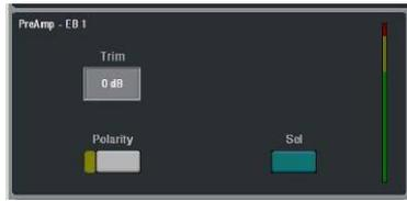
**PREAMP (DUAL MIC/LINE IN)** If the dual input module is detected then the screen includes a touch button to select between the A and B input connections.
