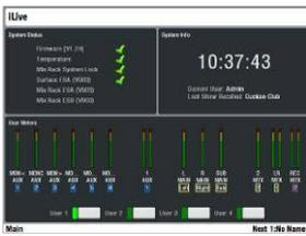
**All screen keys turned off – STATUS** With all the screen keys and strip **SEL** keys turned off the TouchScreen displays the Status page. This shows system status including firmware, temperature, audio system lock and digital audio network status. A **red cross** means a problem is detected. The page also displays the time, current user and last Scene recalled name. The lower part of the screen can be used to select one of the four custom user meter views or the RTA display.
