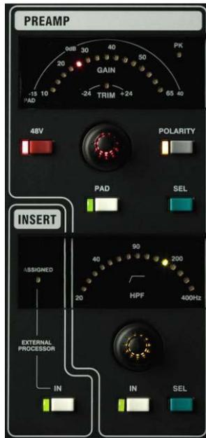
**Note:** To select phantom power using the processing block 48V key hold it down for 0.5 second. This is to protect against accidental operation. Red PP LEDs light on the iLive MIC/LINE input modules when phantom power is detected on their sockets, whether from their own mic preamp or an external sources. These are not available on the T Series.
