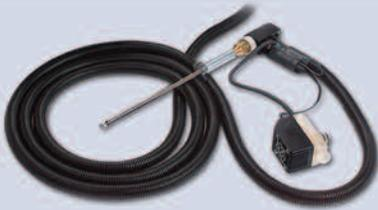
Used in conjunction with the ECA 450, the Flue-Gas Sample Conditioning System functions to remove water vapor from the flue-gas sample, thus preventing the formation of water droplets inside the probe hose. If water droplet were to form, a portion of the gas sample could be absorbed by the water, thus resulting in lower-than-actual NO<sub>2</sub> and SO<sub>2</sub> readings.
