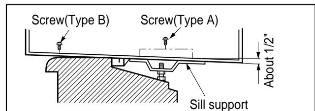
7. Attach the cabinet to the window stool by driving the screws (Type B: Length sixteen millimeters and below.) through the front angle into window stool.
