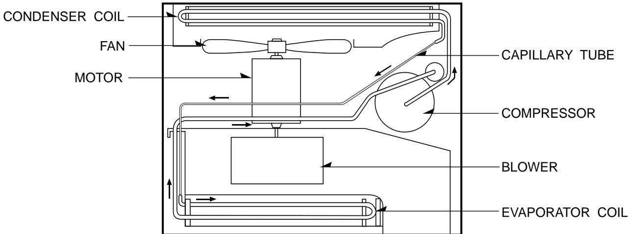
Figure 38 is a brief description of the important components and their function in what is called the refrigeration system. This will help you to understand the refrigeration cycle and the flow of the refrigerant in the cooling cycle.
