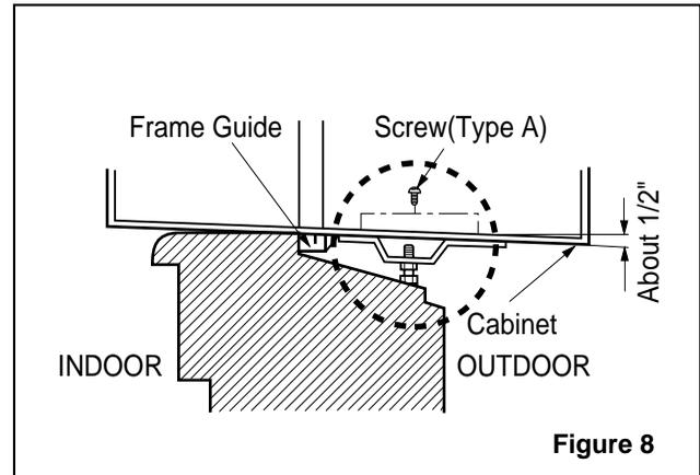
6. The cabinet should be installed with a very **slight tilt(about 1/2") downward** toward the outside (See Figure 9). Adjust the bolt and the nut of Sill Support for balancing the cabinet.
