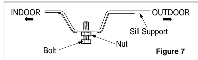
4. Select the position that will place the Sill Support near the outer most point on sill (See Figure 8)
