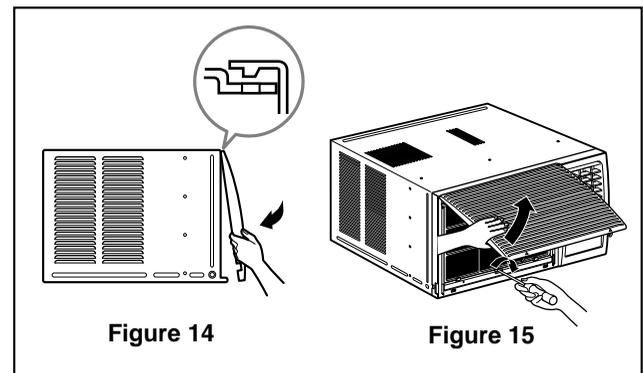
14. Lift the inlet grille and secure it with a Type A screw through the front grille. (See Figure 15)
