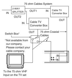
The above cable hook-up allows VCR functions, including viewing one channel while recording another, but it requires two cable TV Converter/Descrambler Boxes, one Switch Box and one 2-Way Splitter.
