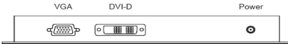
15-pin D-sub VGA and DVI-D
