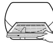
3. Place wet items on top of the rack. Leave space between the items so air can reach all the surfaces. Close the door.
