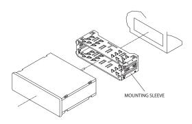
TYPICAL FRONT-LOAD DIN MOUNTING METHOD
