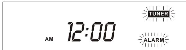
3. While the **ALARM** indicator is flashing immediately press the MEMORY (PROG)/CLOCK ADJ. button. The Hour digits begin to flash.
