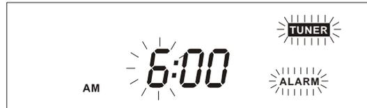
5. Immediately press the MEMORY (PROG)/CLOCK ADJ button. The Minute digits begin to flash. Press the B or F buttons to adjust the display to the correct minute, Example: 6:30 AM, and then press the MEMORY (PROG)/CLOCK ADJ button again.
