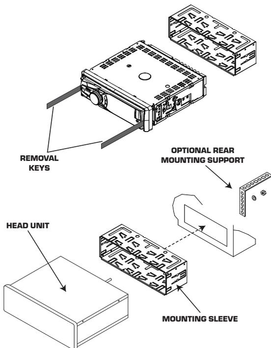
TYPICAL DIN FRONT-LOAD MOUNTING METHOD
