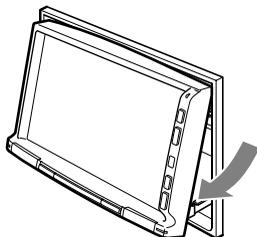
2. When the operation panel is moved to your desired angle, release the button.
