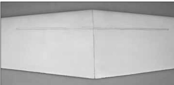
3. Epoxy the foam inserts into the wing slot over the carbon joiner. Make sure they are fully seated against the joiner. The foam inserts may not be completely flush with the bottom of the wing.
