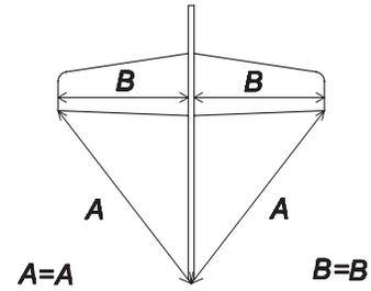
1. Insert the wing into the fuselage. Be sure that the wing is centered and square by making sure all measurements are equal as shown in the sketch.
