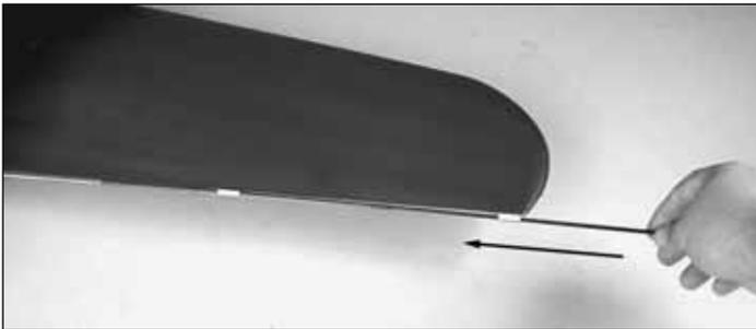
3. Slide the loose carbon rod through the bearings.
