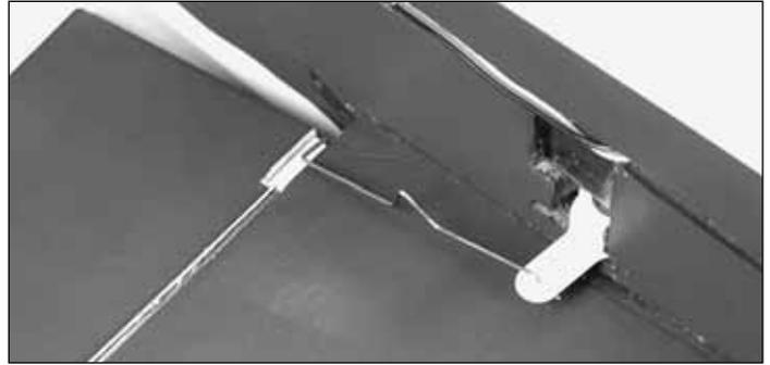
1. Locate the two 2-3/4" [70 mm] prebent **aileron pushrods**. Slightly enlarge the outer hole on the aileron servo arm. Insert the Z-bend end of the pushrods into the outer hole on the aileron servo arm.
