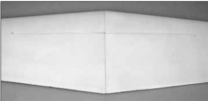
1. Using epoxy, join the two **wing halves** together, making sure to align the root sections.
