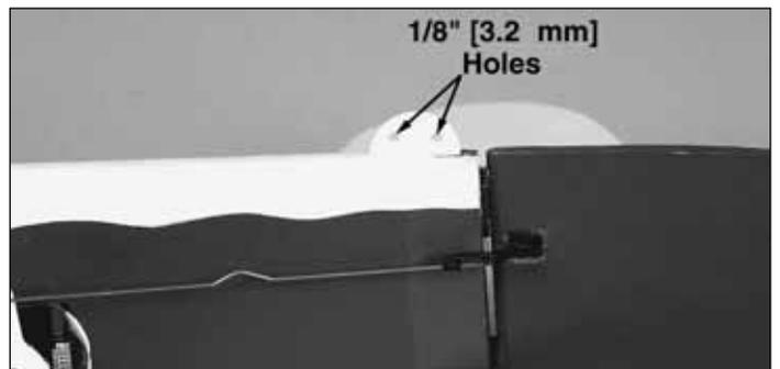
❑ 7. Drill two 1/8" [3.2 mm] holes in the mount. If not flying combat, use the two holes to route the antenna from the receiver.
