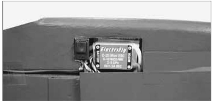
2. Install the ESC as shown using a small section of hook and loop tape. Place the hard "hook" side in the provided cutout in the fuselage and the softer "loop" side on the back of the ESC. If your ESC has a BEC switch, install it in the provided cutout. For some electronic speed controls, it may be necessary to trim the foam slightly to allow for wire clearance and switch mounting.
