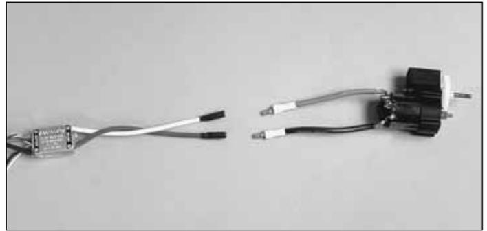
1. Connect the output wires of your ESC to the motor. Check the direction of the motor before permanently installing it.
