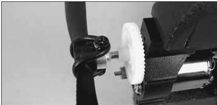
❑ 4. Install the prop saver onto the gearbox output shaft. The screws should seat down into the flat spots on the shaft. Add a drop of thread-lock and be sure the screws are tightened to prevent them from backing out during operation. **Note:** The prop saver has two different diameters. Match the size of your prop hub to the prop saver before installing the prop to the gearbox. Attach the prop using the supplied black O-ring.
