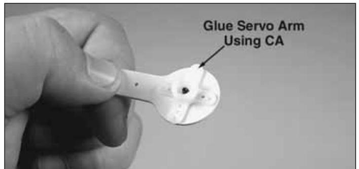
3. Place the original servo arm over the screw, and glue the top of the arm to the extender with CA. Some servo arms have small flanges projecting from the top. If your servo arms have these flanges, sand them off before gluing.
