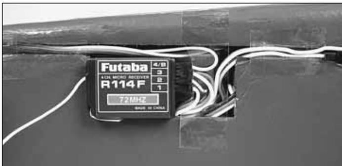
❑ 1. Attach the **receiver** to the cutout in the rear of the fuselage using a small section of the supplied **hook and loop tape**. Place the rough, or “hook” side of the tape into the cutout in the fuselage and the soft “loop” side of the tape on the back of the receiver.
