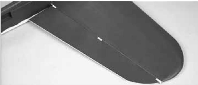
4. Test fit an aileron onto the carbon rod as shown. If satisfied with the fit, glue the aileron to the carbon rod using CA. DO NOT glue the aileron to the bearings. The rod must freely rotate in the bearings, so the aileron must only be glued to the carbon rod.
