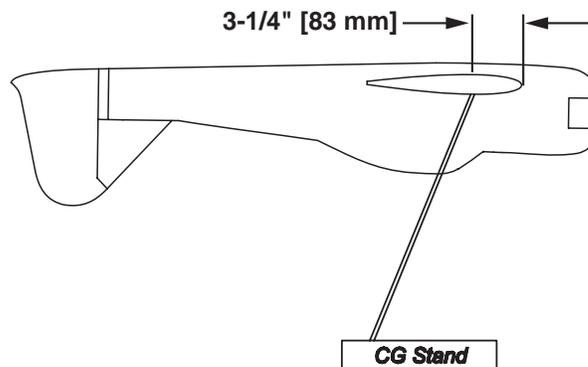
2. With the wing attached to the fuselage and all parts of the model installed (ready to fly), place the model upside-down on a Great Planes CG Machine, or lift it upside-down at the balance point you marked.
