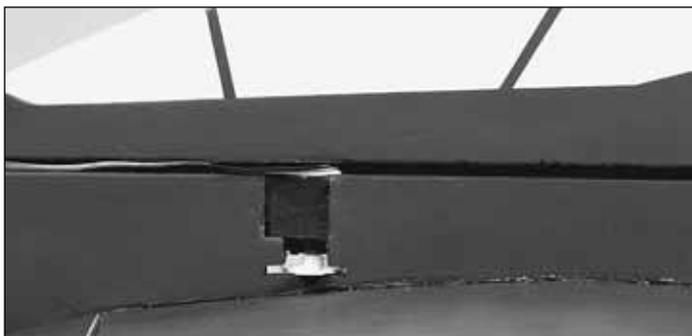
6. Center your aileron servo with your radio and screw the extended double-sided arm onto the servo. When you glue the extended servo arm, be sure it is exactly centered as shown. Epoxy the aileron servo into the cutout in the fuselage.
