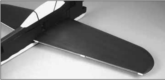
2. Test fit one of the wing hinges in the wing. The outer bearing should be flush with the wing tip. When satisfied with the fit, epoxy the hinge in place. Be careful to avoid getting epoxy into the open bearings.
