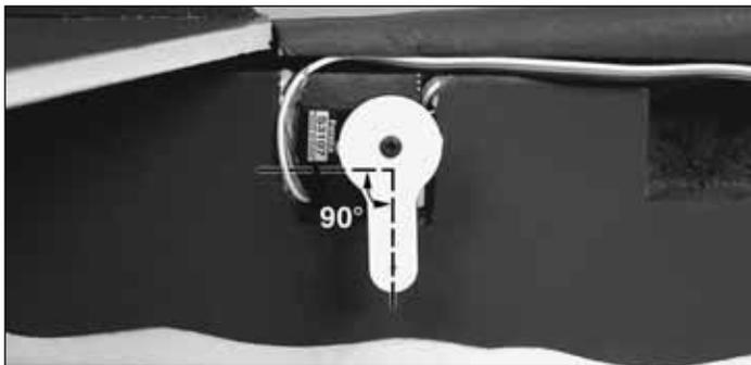
5. Epoxy the other tail servo into the cutout from the right side of the plane side with the output shaft toward the front. Center the servo with your radio and screw the extended arm onto the output shaft with the arm oriented straight down.
