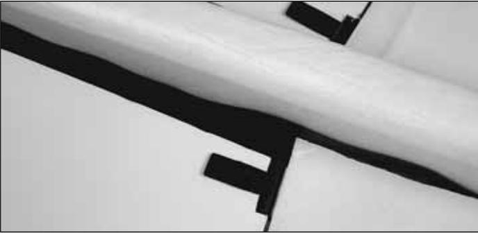
5. Apply a small spot of foam-safe CA to the bottom of the control horn and insert it into the cut in the aileron. Press a nylon **backplate** on the backside of the control horn as shown.
