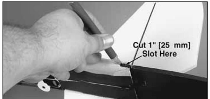
❑ 5. Cut a 1" [25 mm] slot in the bottom of the fuselage at the tail as shown. The exact location is not important; it simply needs to be at the tail of the fuselage. Do not attach the mount to the rudder control surface.
