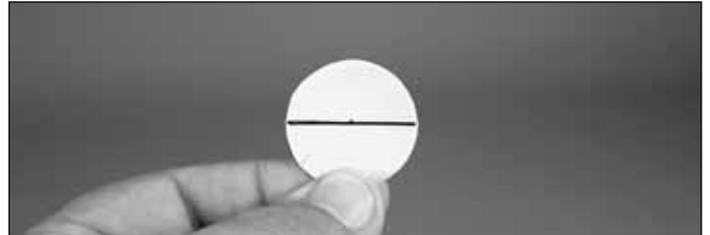
❑ 4. Locate the 1" [25 mm] plastic streamer mount. Mark the approximate midpoint of the mount.
