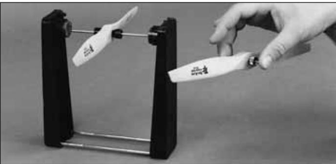
Carefully balance your propeller and spare propellers before you fly. An unbalanced prop can be the single most significant cause of vibration that can damage your model. Not only will motor mounting screws and bolts loosen, possibly with disastrous effect, but vibration may also damage your radio receiver and battery. When balancing the propeller that came with your Fun Force ARF, add tape to the light side of the propeller. Do not shave material away as is done with traditional propellers.
