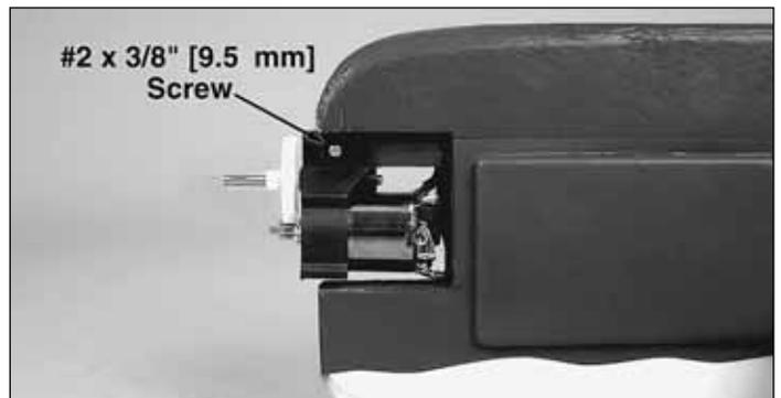
3. Slide the gearbox onto the square **wood stick** in the nose. Secure it with the supplied #2 x 3/8" [9.5 mm] **screw**.
