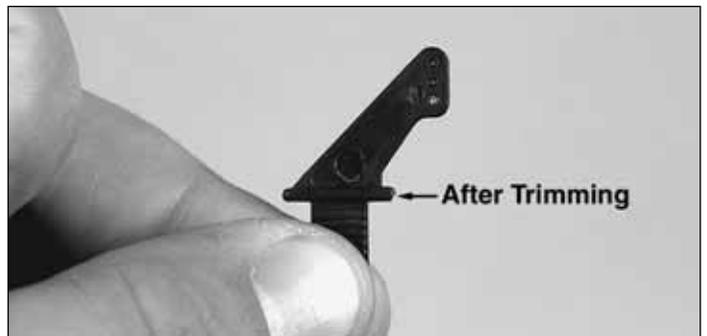
3. Locate a black nylon **control horn**. Trim the small plastic section away as shown.
