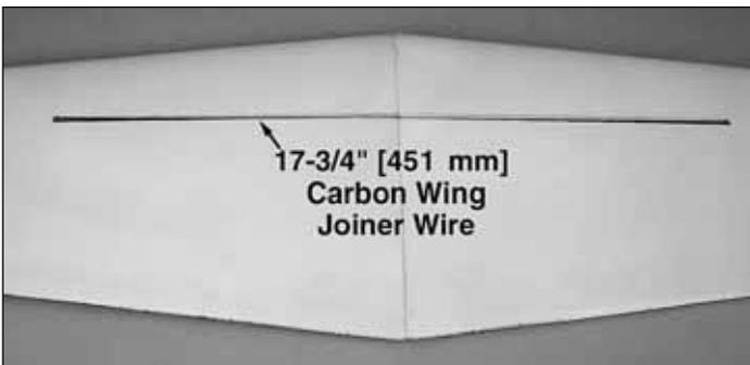
2. Epoxy the 17-3/4" [451 mm] carbon **wing joiner tube** into the slot on the bottom of the wing. Make sure it is fully seated in the slot.
