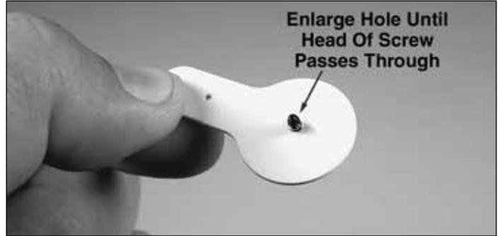
1. Remove the screws and servo arms from all of your servos. Enlarge the hole in the center of the extender until the head of the servo screw fits through.
