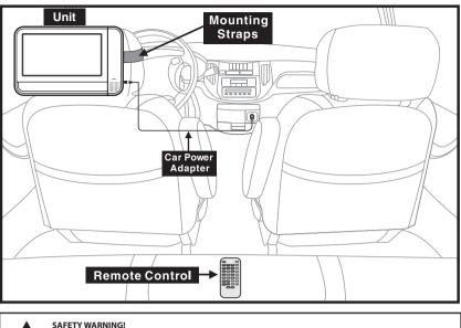
This unit should never be used by the vehicle's driver or left unsecured in the vehicle while driving If this unit is being used in your vehicle, be sure that it is secured or held safely, and does not obstruct any safety device, including air bags or seat belts.
