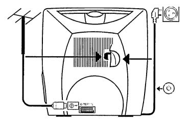
1 Insert the aerial plug into the Tr socket.
