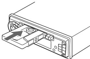
If a cassette is already inserted, press **FNC** repeatedly to select Tape Play mode to start playback. Playback starts in the direction that the unit played back previously.
