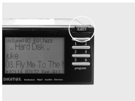
1. Push the "EJECT" button to eject the front panel.
