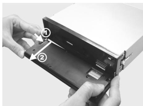
2. Hold the front panel and push to right side, and remove the front panel.
