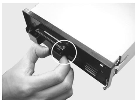
3. Press the left side of the HDD enclosure and take it out.
