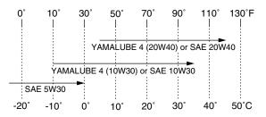
Recommended engine oil grade: API service SE, SF, SG type or higher Engine oil quantity:
