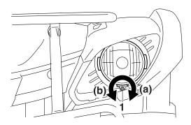
1. Headlight beam adjusting screw
