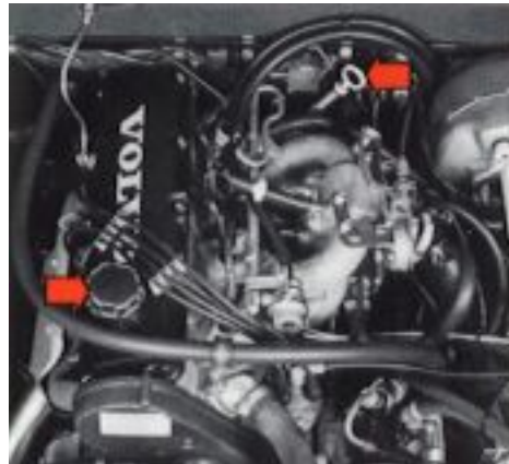
Checking oil level
