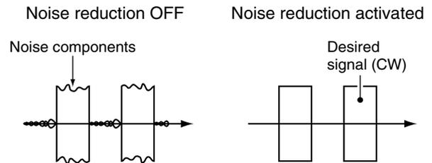
Higher setting of the [NR] level results in audio signal masking or distortion. Set the [NR] level for maximum clarity. The noise reduction function is available in all modes.
