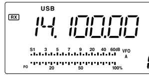
Rotating the tuning dial changes the frequency in 10 Hz steps.
