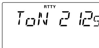
RTTY mark frequency is set to 2125 Hz. 2125, 1615 and 1275 Hz are available.
