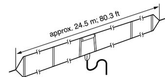
Covers from 1.9–30 MHz bands. Has an SO-239 connector. 30 m (98.4 ft) coaxial cable with PL-259 connector is supplied.
