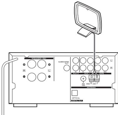
Place the antenna on a shelf or hang it on a window frame, etc., in the direction which gives the best reception. Keep all other wires such as power cords, speaker wires or interconnect wires as far away as possible from the antenna.
