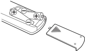
1. Remove the battery compartment cover.
