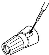
Make sure none of the wire insulation is under the terminal, only the bare, stripped wire.
