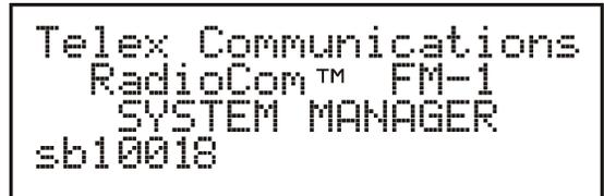
The lower left-hand corner contains the software version in the FM-1. After the start-up screen the event screen will be displayed. The event screen is the main default screen. It will display the current event in FM-1 memory. Up to 99 events may be stored in the FM-1 and on a card, see the "FM-1 Menu Flow Chart section for the menu structure.
