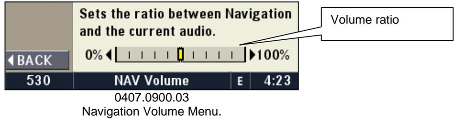
Change the volume ratio between audio source and navigation voice by turning the VOL rotary knob.
