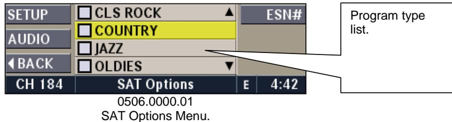
Select one of the desired program types by turning the OK knob and confirming the selections by pressing the knob.
