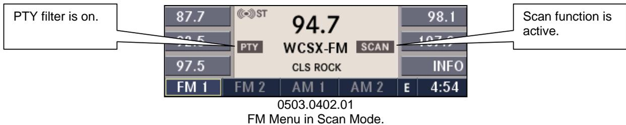
The radio is now scanning through all available stations with the selected program types. Press the **SCAN** button again to stop the scan function and to select the currently playing radio station.
