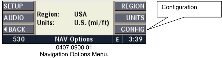
Press the CONFIG multifunction button to display the Navigation Configuration Menu.
