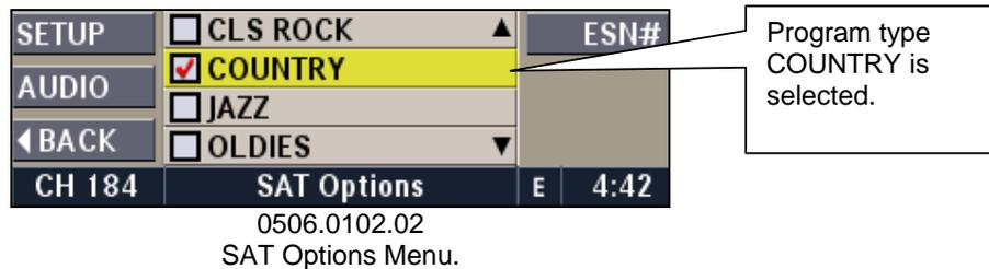
Press the **SCAN** to start the scan function. You must start SCAN from this PTY screen to scan by PTY.
