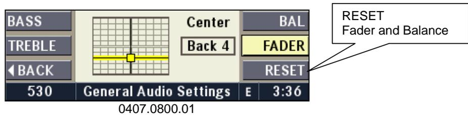
**Note:** The RESET multifunction button in the Tone Menu takes effect for the balance and fader settings for all audio sources. The BAL or the FADER multifunction button has to be activated before pressing the RESET multifunction button.
