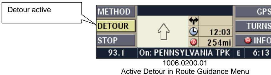
Press the DETOUR multifunction button to access the Detour Menu, while the detour function is active.
