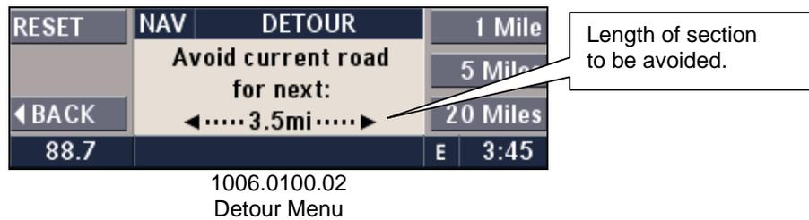
Set the length of the section to be avoided by turning the OK knob or press one of the 1 Mile, 5 Miles, or 20 Miles multifunction buttons.
