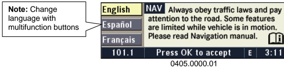
The disclaimer will be activated in the navigation mode after the ignition was turned on.
