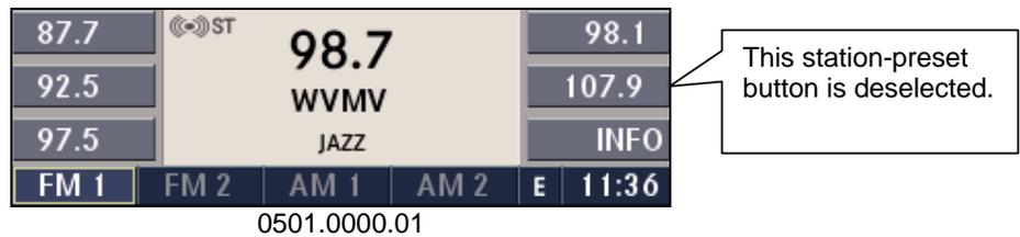
In order to store the desired station, press one of the station preset buttons for more than 3 seconds. You will also see the radio station stored in the highlighted multifunction button symbol and PRESET is displayed in the upper right corner of the screen.
