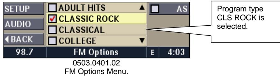
Press the **SCAN** button to start the scan function. You must start SCAN from this PTY screen to scan by PTY.
