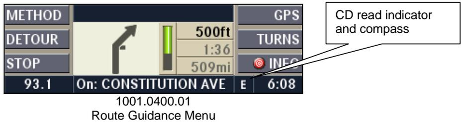
After this indicator disappears, the radio and internal disc player are available for their normal use. If the navigation needs additional information to recalculate a new route, the user receives a voice prompt to reinsert a navigation CD and the CD read indicator turns red until the CD is inserted.
