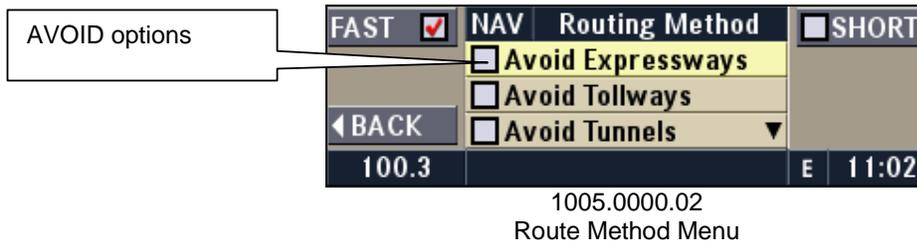
The current avoid items are displayed. To change the options, press the AVOID multifunction button in the Routing Method Menu.
