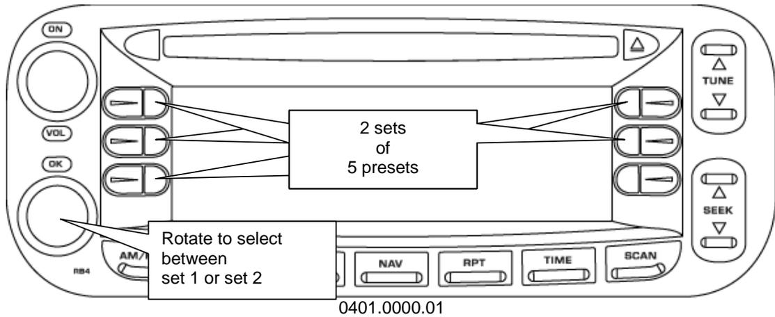
You can access the second set of station preset buttons by turning the OK knob to toggle between the FM1 and FM2 sets.
