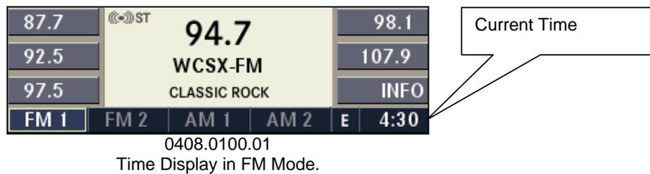
Press the **TIME** button to display the time in the main display.
