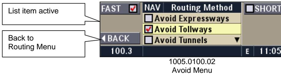
Press the multifunction buttons of the items to avoid and press the ◀BACK multifunction button to return to the Routing Method Menu.
