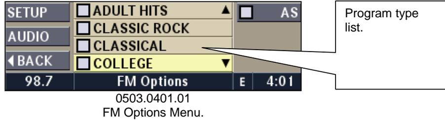
Select one or more of the desired program types by turning the OK knob and confirming the selections by pressing the knob.
