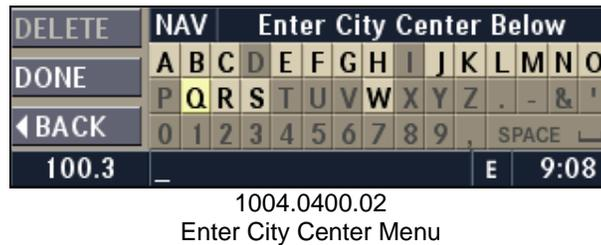
Enter a city center name by turning the OK knob and press the OK knob in to confirm your selection.
