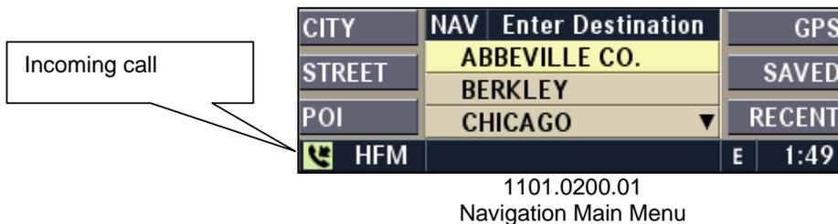
If the navigation radio is in any other mode or if you press the **MODE** button during an incoming call, the information transmitted by the cell phone is displayed in the HFM (Hands-Free Module) Menu.
