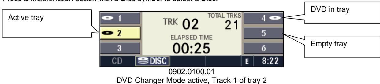
**Note:** The currently selected Disc tray number is displayed in Navigation Mode also. "1TRK2" indicates the Disc Changer Mode is playing track 1 from the Disc in tray 2.
