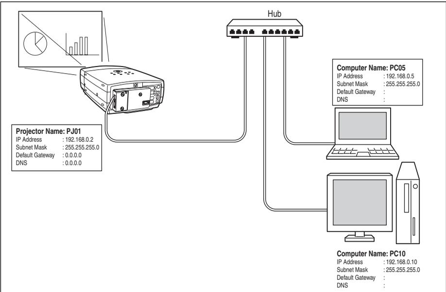
When the projector is connected to the computer directly without hub, the UTP cross cable should be used .
