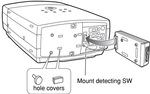
**3** Tighten three screws by using a coin etc.
