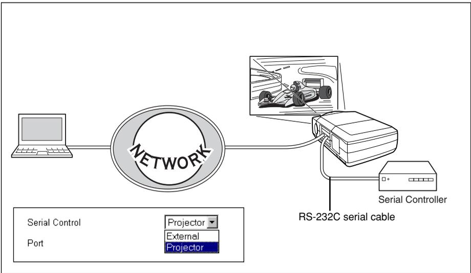
☞ When connecting the peripheral equipment to this Network Unit, you should notice the type of serial cables. This product provides a reverse (cross) type of serial port. When connecting the peripheral equipment, please use an optimum serial cable according to the polarity of the port on the equipment. For further pin allocation please see the Port Specification on page 78.
