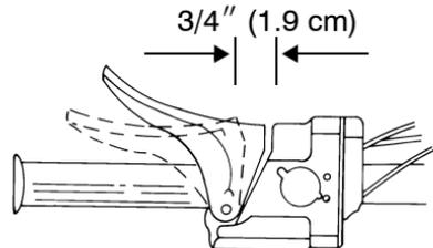
If the distance is greater than this recommendation, the brake cable must be adjusted.
