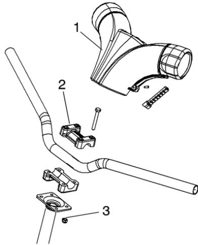
3. Adjust the handlebar to the desired height. Be sure handlebars, brake lever and throttle lever operate smoothly and do not hit the fuel tank, windshield or any other part of the machine when turned fully to the left or right.
