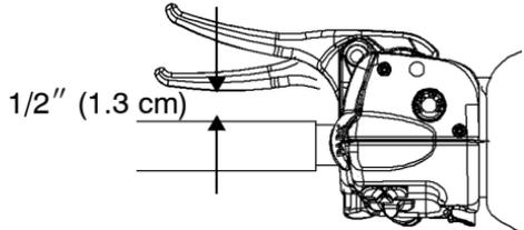
**NOTE:** If the brake lever feels “spongy” when squeezed, check the brake fluid level and condition. Add fluid as needed. See page 104.
