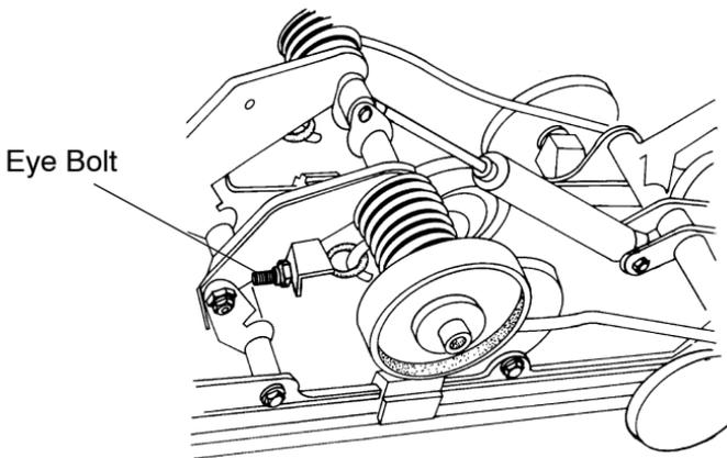
**NOTE:** Rear spring settings will affect ski-to-ground pressure. If ski pressure is too light it may be desirable to tighten the rear springs for an increase in ski-to-ground pressure.
