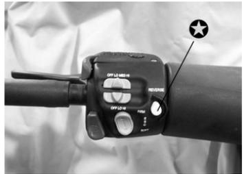
**NOTE:** The maximum engine RPM will be 6000 when in reverse.
