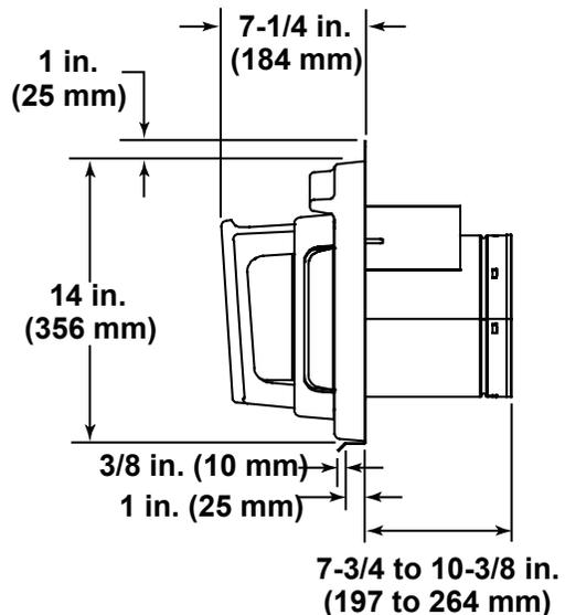
Figure 14.4 SLP Series Vent Components
