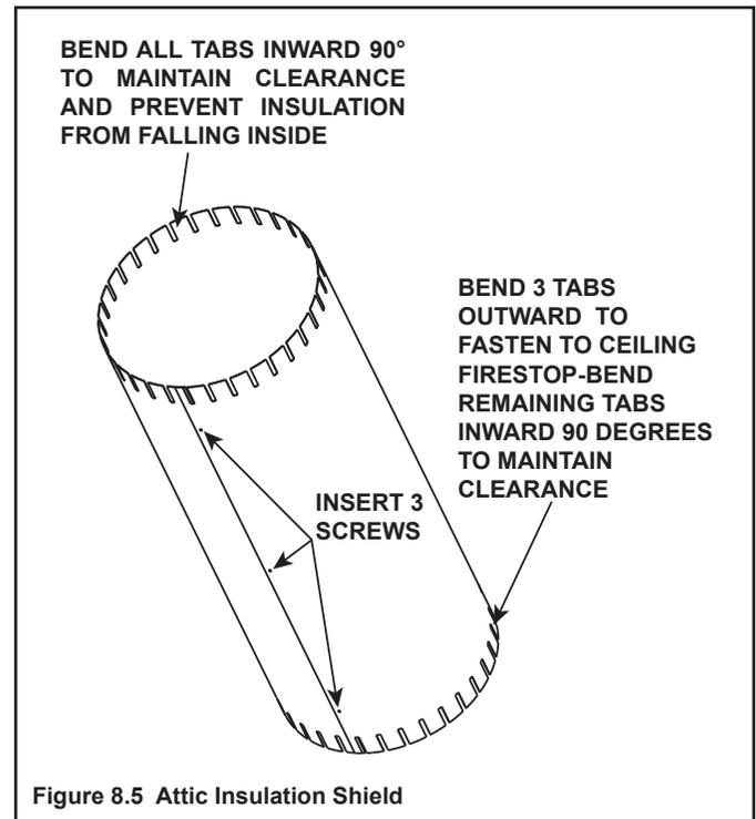
Figure 8.5 Attic Insulation Shield
