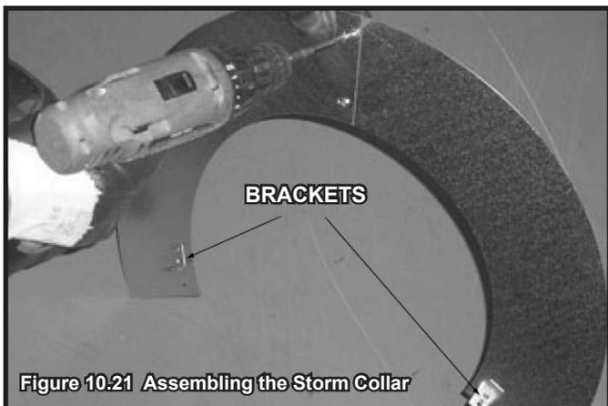
Figure 10.21 Assembling the Storm Collar
