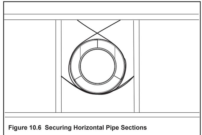
Figure 10.6 Securing Horizontal Pipe Sections
