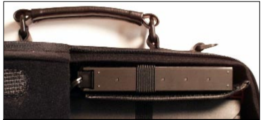
Correctly Installed Battery
