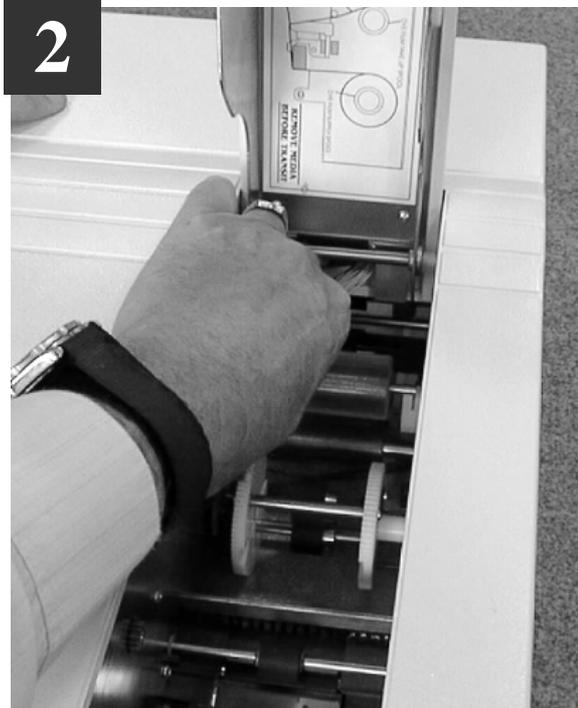
**Remove the 'tacky' roller before each batch of 100 cards, by putting your fingers beneath it and "snapping" out the left hand end of the roller. Remove surface dust by using a strip of 'Scotch' adhesive tape, and "snap" back into place.**
