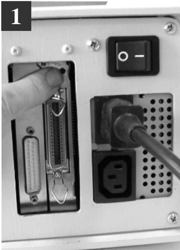
**1** At the rear of the printer, locate the TEST Push-button. This is located in the rear panel, just above the Centronics parallel interface connector. Press the push-button momentarily.
