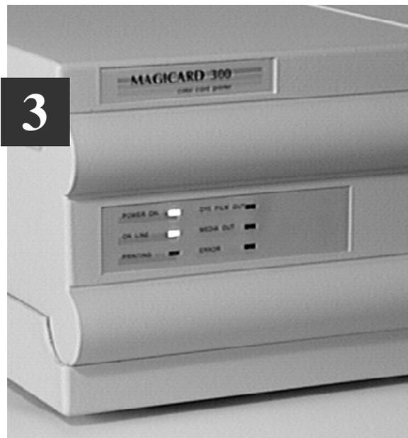
3 Switch ON. The indicators should all flash and the motors run briefly. Finally, the POWER ON and ON LINE indicators will remain ON..
