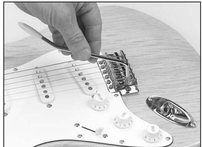
**Figure 37.** Installing the tremolo arm.
