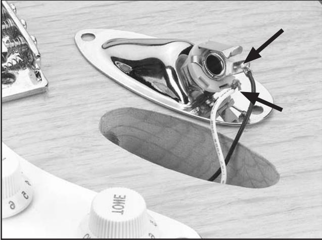
**Figure 27.** Soldered audio wire.
