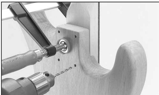
**Figure 14.** Drilling the screw holes.
