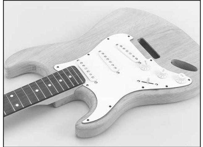
**Figure 18.** Pick guard alignment.
