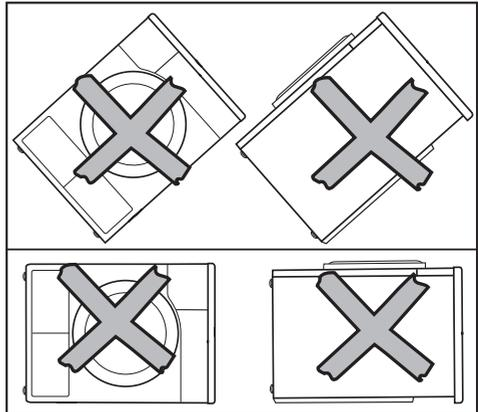
**⚠** If the tumble dryer has not been transported as described, then it must be left to stand for at least 1 hour before it is connected to the electricity supply. Otherwise the heat pump can be damaged.
