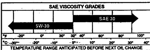
**NOTE:** Although multi-viscosity oils (5W30, 10W30 etc.) improve starting in cold weather, these multi-viscosity oils will result in increased oil consumption when used above 32°F. Check your engine oil level more frequently to avoid possible engine damage from running low on oil. Change the oil after every 25 hours of operation or at least once a year if the tractor is not used for 25 hours in one year.
