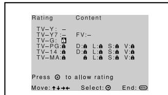
To unblock a rating, select it by moving the joystick up or down, then press
