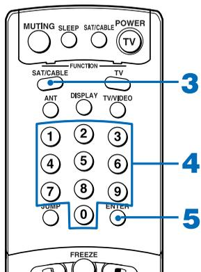
From the “Manufacturer’s Codes” listed on page 73, select the three-digit code number for the manufacturer’s code for your component. If more than one code number is listed, start with the number listed first. Use the code number to complete the following procedure.
