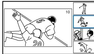
**3** To enlarge the selected channel into the left frame, press
