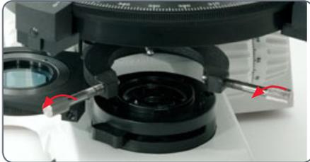
5. Slide the substage condenser into the fork mount located underneath the stage by aligning the positioning pin on the condenser into the slot on the back of the fork.
