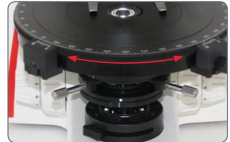
4. Loosen the stage brake and rotate the stage until the noticeable point of the sample is furthest away from the center of the crosslines. This may even be outside of the field of view. This indicates the objective is not centered to the stage.
