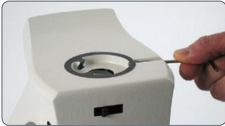
2. Align the shape of the polarizing viewing tube with the shape of the module.
