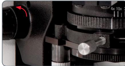
7. Tighten the thumbscrews to roughly center the substage condenser so that the top lens of the condenser is centered beneath the objective in use. You will more accurately center and focus the condenser when you reach section Koehler Setup.
