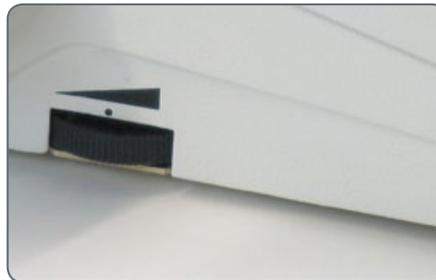
4. Turn on the microscope using the switch on the bottom right-hand side of the microscope stand.
