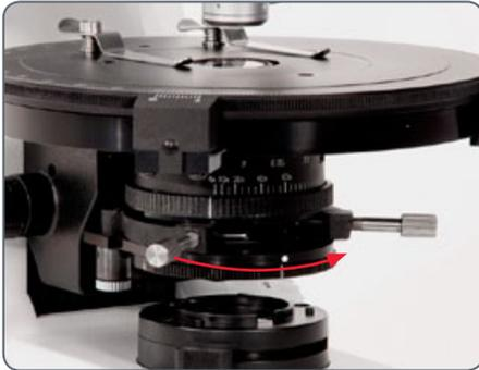
1. Loosen the polarizer locking thumbscrew, which is located on the right-hand side of the polarizer.
