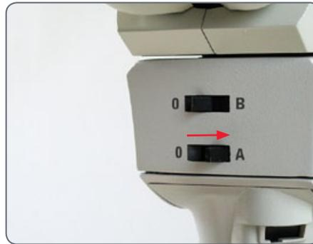
4. Increase the illumination intensity slightly. You will notice while looking into the microscope with the Polarizer and Analyzer in place and no specimen, that the field will look dark. If not, rotate the polarizer slightly until you have the darkest field of view.
