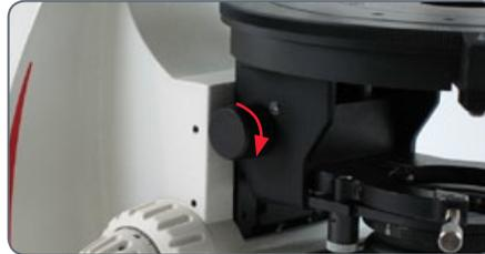
3. Swing the polarizer, which is connected to the bottom of the condenser mount, to the left.
