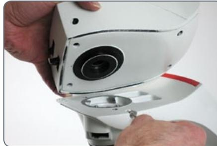
3. Insert the dovetail of the module into the stand. (Analyzer/Bertrand Lens Module shown).
