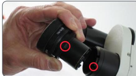
5. If you wear eyeglasses for microscope viewing, keep the rubber eyeguards folded down. If you do not wear eyeglasses, you may find it useful to unfold the rubber eyeguards in order to block out ambient room light.
