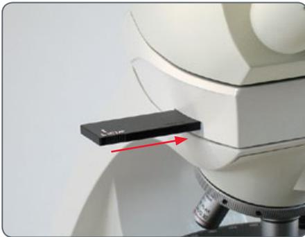
3. If you have an Analyzer/Bertrand Lens module, swing in the Analyzer by flipping the lower rocker of the module to the right (the "A" position/Analyzer in), while ensuring the upper rocker of the Analyzer/Bertrand Lens Module is flipped to the left (the "O" position/Bertrand Lens out).
