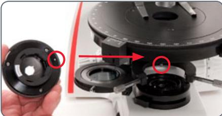
6. Raise the condenser to its highest position using the condenser focus on the left-hand side of the substage
