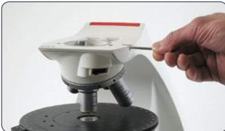
2. Align the shape of the module with the shape of the microscope stand.
