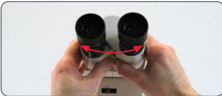
**i** The viewing tubes maintain a constant tube length for all interpupillary settings. This means that a change of interpupillary distance does not affect parfocality, magnification, or calibrations that depend on magnification.
