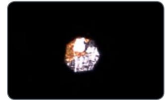
2. Use the condenser focus knob on the left-hand side of the substage to bring the leaves of the field diaphragm into sharp focus.
