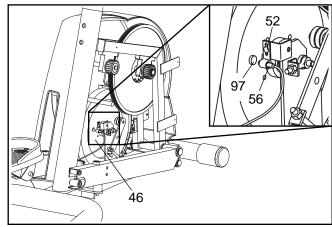
Turn the Flywheel (46) until the Magnet (97) is aligned with the Reed Switch (56) (refer to the inset drawing). Loosen the indicated Screw (52). Slide the Reed Switch slightly closer to the Flywheel, and retighten the Screw. Make sure that the Magnet will not hit the Reed Switch when the Flywheel turns. Repeat until the console displays correct feedback.
