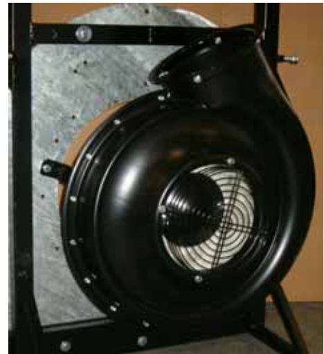
Ø500 fan with multiplier, 2-speed plus neutral.
