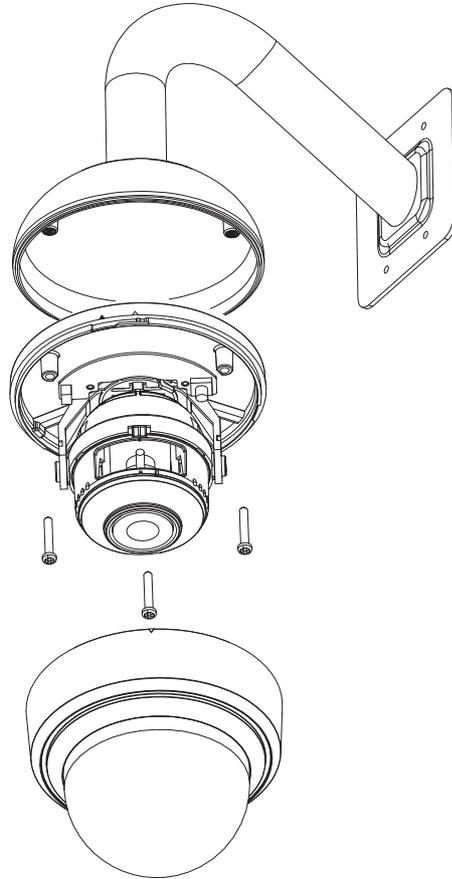
**Figure 3.1** Wall Mount installation
