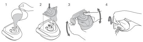
Wash the water chamber, tub plate and tub plate seal in warm water, using a mild detergent. Use the yellow cleaning plug to assist in the cleaning process (see steps 1 to 4). Rinse thoroughly in clean water and allow them to dry away from direct sunlight.
