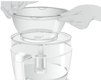
2. Fit the mini blade on the power shaft. It may be necessary to rotate the blade until it falls into place. The mini bowl can also be placed in the chef's bowl in a similar manner.
