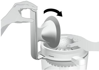
**NOTE:** Use of the citrus press without the clip-on lever arm is not recommended. If you do use it without the lever arm, remove the lever arm from the basket (see step 14).
