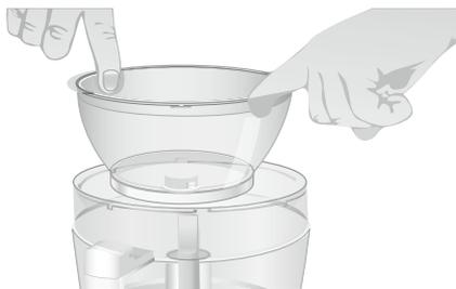
6. Turn the work bowl to the left to unlock it from the base. Lift to remove.
