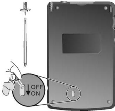
**IMPORTANT:** Keep the battery switch set to ON (down position) unless you need to restore factory defaults.
