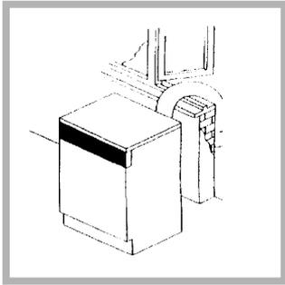
1. The end of the tube should be directed downwards, to prevent warm moist air from condensing in the room or in the dryer.
