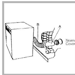
1. Leave an opening in the wall to the left of the dryers proposed position.
