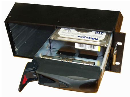
Figure 6-2 Drive Inserted half way in to System
