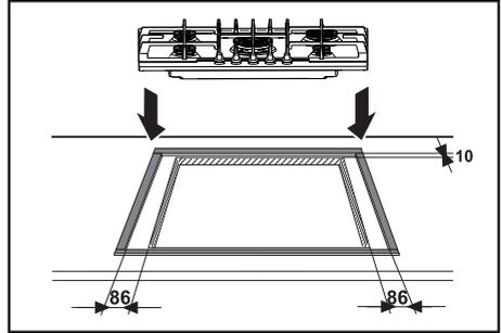
The edge of the hob forms a double seal which prevents the ingress of liquids.
