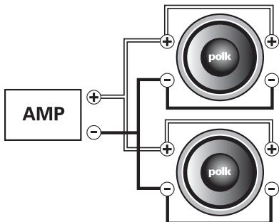
With coils and speakers wired in parallel, two dual 4 Ohm speakers will present a 1 Ohm load. (Not recommended unless amplifier is rated for 1 Ohm operation.)
