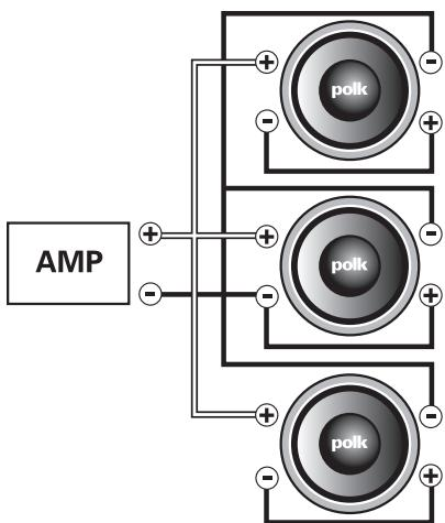
With the coils wired in series and the speakers wired in parallel, 3 dual 4 Ohm speakers will present a 2.7 Ohm load.
