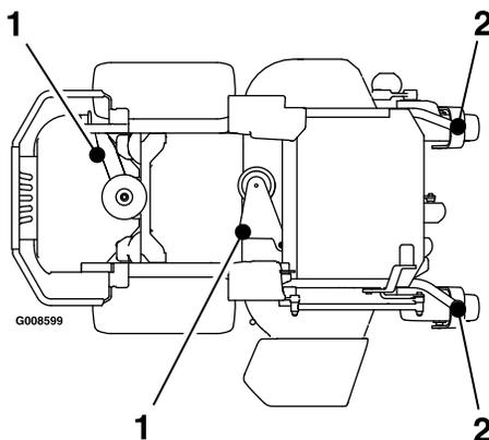
3. Lubricate front caster pivots once a year. Remove hex plug and cap. Thread grease zerk in hole and pump with grease until it oozes out around top bearing. Remove grease zerk and thread plug back in. Place cap back on.
