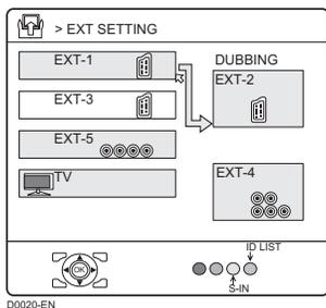
**2 Press the yellow button and set the S-IN (S-VIDEO input). Then press the OK button**
