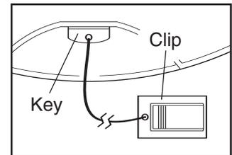
Insert the key fully into the console. After a moment, the displays will light. **Test the clip by carefully taking a few steps backward until the key is pulled from the console. If the key is not pulled from the console, adjust the position of the clip.**
