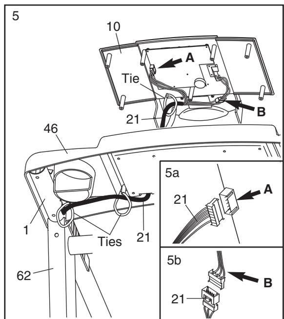
6. Set the Console (10) in the Console Base (46). **Be careful to avoid pinching any wires.** Insert the excess Wire Harness (21) into the large hole in the side of the right Handrail (1). **Securely tighten the plastic ties on the bottom of the Console Base to prevent the Wire Harness from slipping.** Cut off the ends of the plastic ties.
