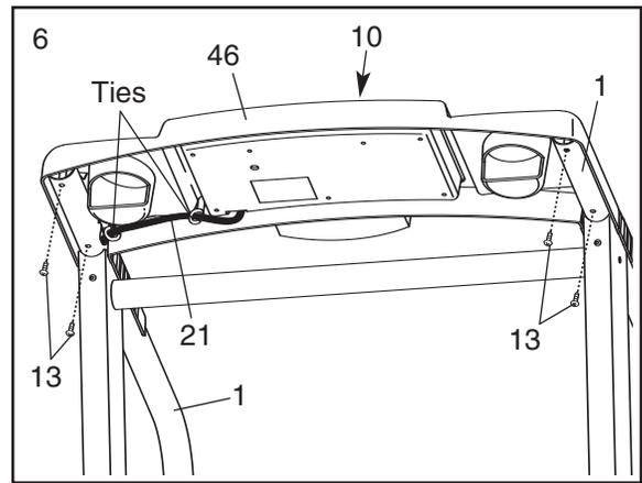
7. Attach the Console (10) to the Console Base (46) with seven 3/4" Screws (13). **Make sure that no wires are pinched. Start all seven Screws before tightening them; do not overtighten the Screws.** Note: Make sure the indicated 3/4" Screw is not overtightened. Overtightening the Screw may cause the Console to not function properly.
